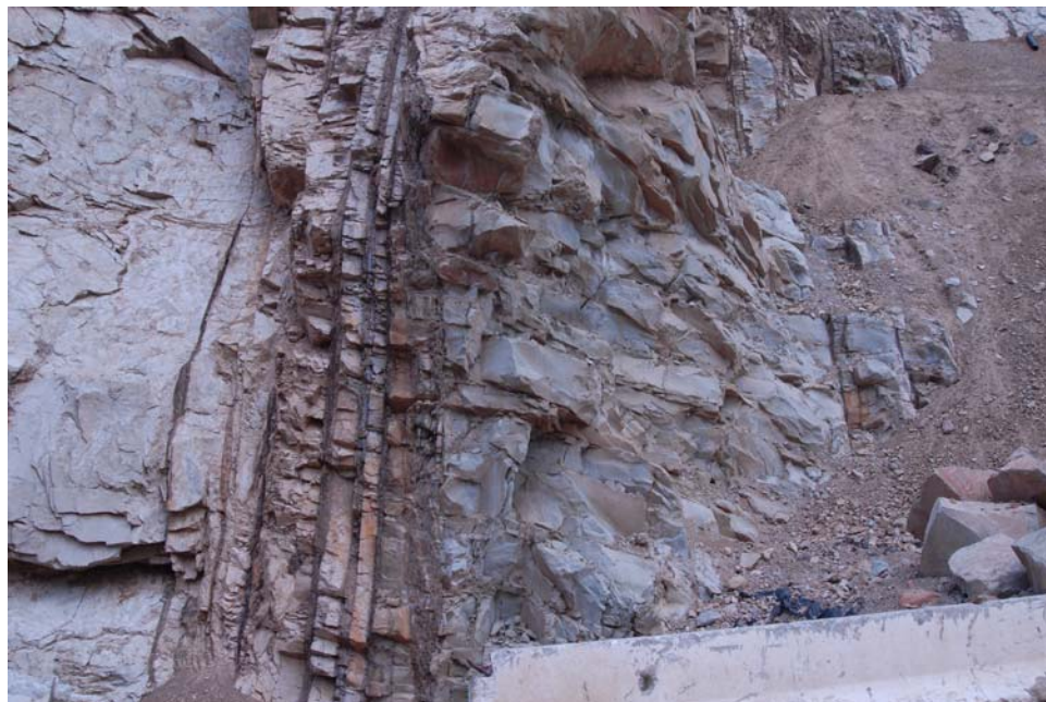
Photo 10: Jointing patterns in Domain A sandstones.
