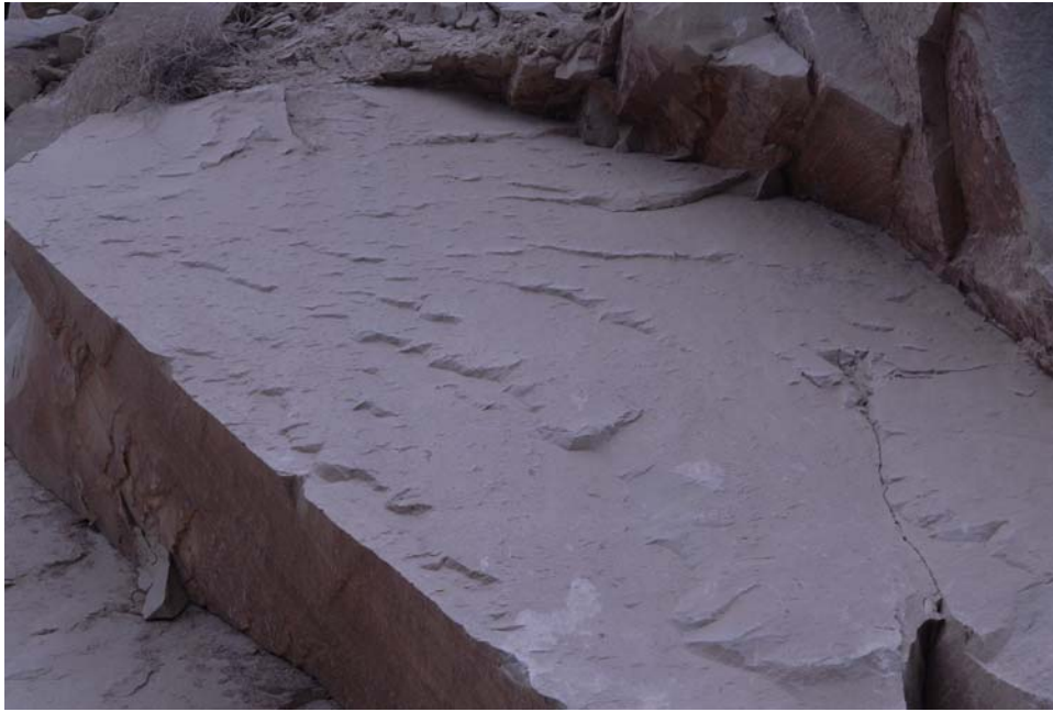
Photo 11: A joint surface in Domain C sandstones.
